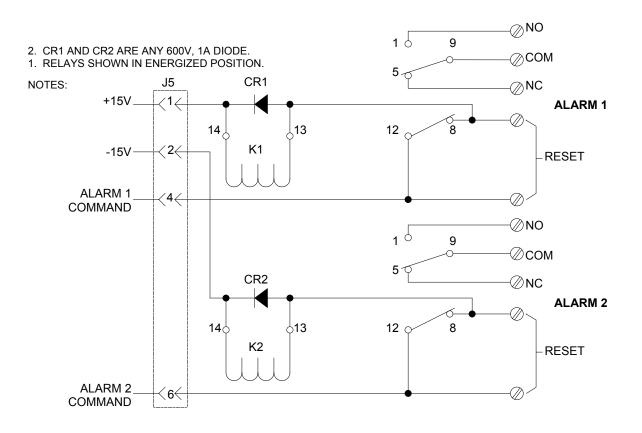
Figure 3-4. Schematic Circuit of Alarm Relay Assembly
